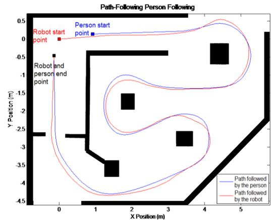
Fig. 2. Example of a path-following algorithm.
