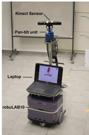
Fig. 1. The robotic platform.
