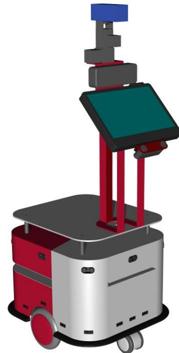
Figure 3. Customised robuLAB10 platform
