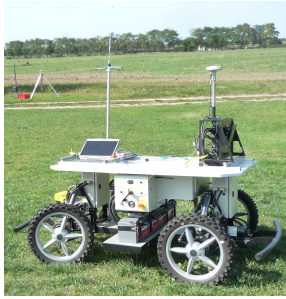
Fig. 3 RobuFAST A on site with its DGPS fixed base (upper left hand side)
