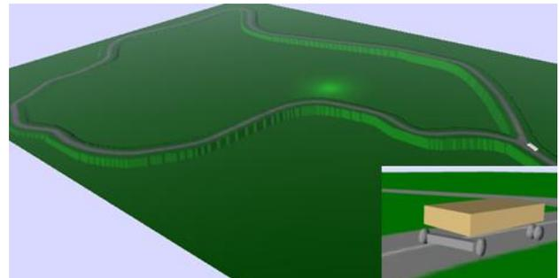
Fig. 19: 3D model automatic generation using recorded GPS trajectories
