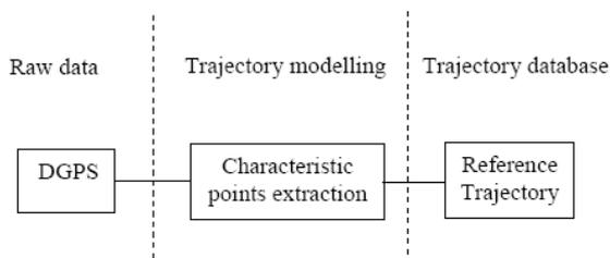
Fig. 7. Teach by showing trajectories recording.
