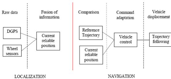
Fig. 8. The autonomous navigation process.
