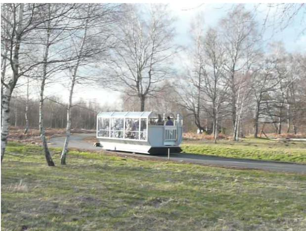
Fig. 20: Vulcania volcanBUL Grand Opening, using the GPS-controlled driverless robuRIDE transporting 28 persons at 8km/h.
