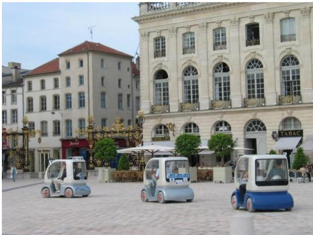
Fig. 11. Platooning of cybercars.
