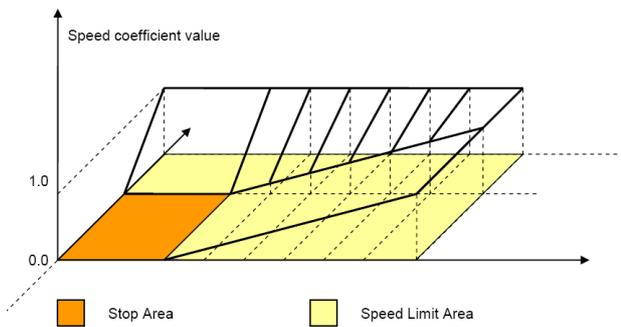
Fig. 10. Obstacles detection and vehicles speed adjustment.
