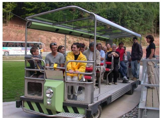
Fig. 13. Simserhof Entertainment park. Cybercars using embedded wires.
