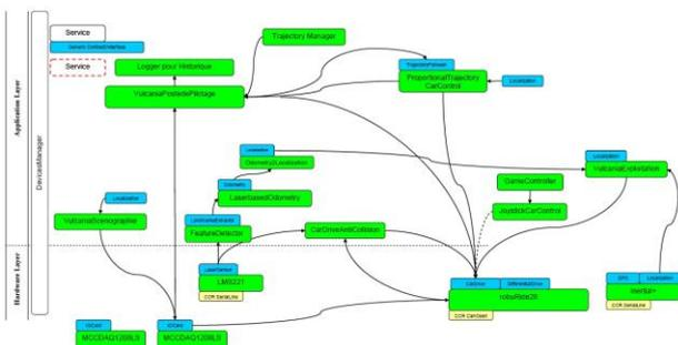
Fig. 17: Vulcania robuBOX control architecture
