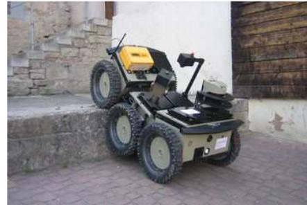
Fig.7. RobuBOX-Outdoor implemented on a robuROC6.
