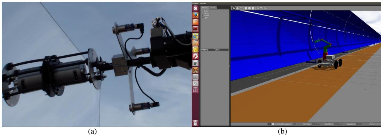
**FIGURE 6.** Robot placing the reflectometer on the mirror (a) and simulation environment (b)
