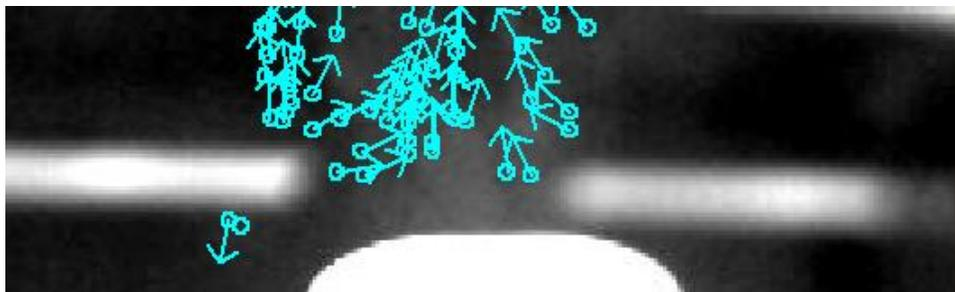
**FIGURE 5.** Optical flow used to detect steam
