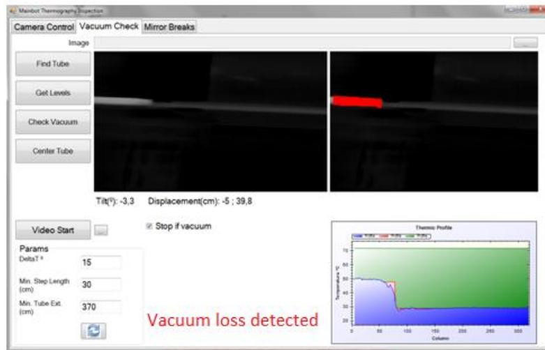
**FIGURE 3.** Application developed for vacuum loss detection
